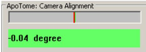
Once the camera has been aligned with sufficient precision, please lock the camera adapter in this position.
