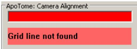
In this case the deviation of the grid lines from the camera horizontal is probably too great. Rotate the camera until the long side of the camera's field of view is roughly parallel to the grid lines. To do this, loosen the corresponding lock on the camera adapter and realign the camera.
