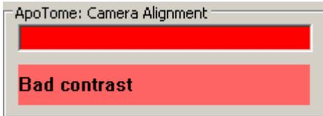
In this case you should take steps to increase the contrast (e.g. increase the exposure time, refocus the grid (step 3)).
