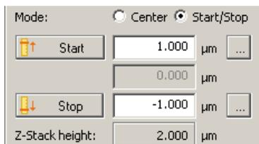
The alternative way to define the focus range is **Start/Stop** mode. In this case you should move the microscope to the top and bottom of the range and then click on the **Start** and **Stop** buttons. These have deliberately not been called 'top' and 'bottom' as it doesn't matter whether you enter the top position as *Start* and the bottom position as *Stop* or vice versa.
