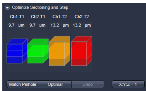
Fig. 5-42 Optimize Sectioning and Step: Optimal Interval is set starting with one Airy unit for all channels
